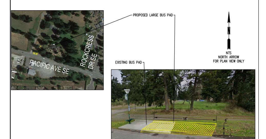
EXISTING CONDITION: BUS STOP WITH SIMME SEAT ON AN ELEVATED PAD WITH A RAMP.
