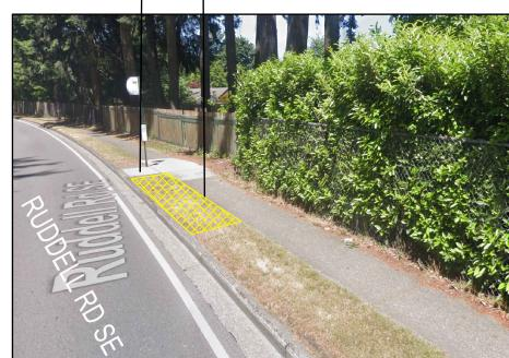
EXISTING CONDITION: 3' X 5' BUS STOP WITH SHELTER AND 5' WIDE SIDEWALK. INSTALL: 3' WIDE BUS PAD (APPROX. 19' X 3'). MATCH EXISTING TOP OF CURB AND SIDEWALK. SEE SHEET L-DT-01 FOR LARGE PAD DETAIL. NOTE: PROTECT EXISTING TREE
