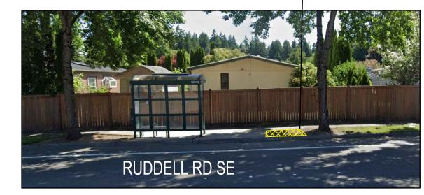
EXISTING CONDITION: BUS STOP PAD (APPROX. 19'X4.5') WITH SHELTER, 5.5' WIDE SIDEWALK, AND 4.5' WIDE PLANTING STRIP. INSTALL: BUS PAD (APPROX. 5'X4.5') SOUTH OF EXISTING PAD TO MEET LARGE PAD REQUIREMENTS. MATCH EXISTING TOP OF CURB AND SIDEWALK.
