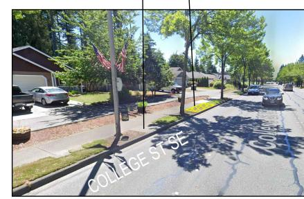
EXISTING CONDITION: BUS STOP PAD (APPROX. 4'X5'), SIDEWALK, AND 4' WIDE PLANTER STRIP. INSTALL: REAR BUS PAD (APPROX. 4'X6'). SEE SHEET L-DT-01 FOR REAR BUS PAD DETAIL NOTE: PROTECT EXISTING LIGHT POLE AND TREES.
