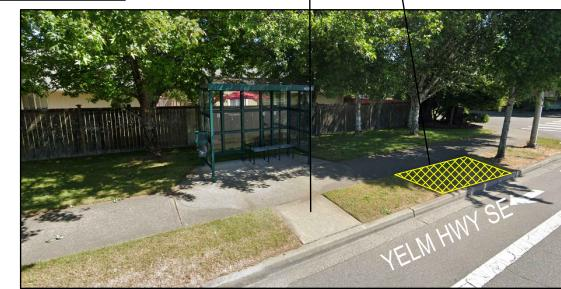
EXISTING CONDITION: BUS STOP WITH SHELTER, EXISTING BUS PAD (APPROX. 4.5'X4.5'), 6' WIDE SIDEWALK, AND 4.5' WIDE PLANTER STRIP.
