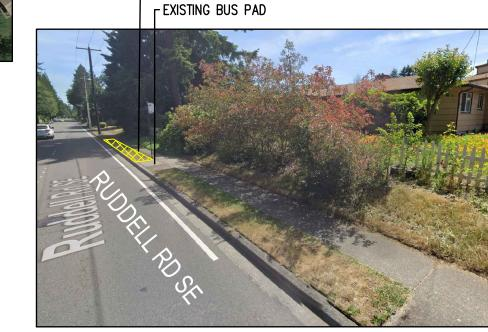
EXISTING CONDITION: BUS STOP PAD (APPROX. 6'X3'), 5' WIDE SIDEWALK, AND 3' WIDE PLANTER STRIP. INSTALL: LARGE BUS PAD (APPROX. 18'X3'). MATCH EXISTING TOP OF CURB AND SIDEWALK. SEE SHEET L-DT-01 FOR LARGE PAD DETAIL.
