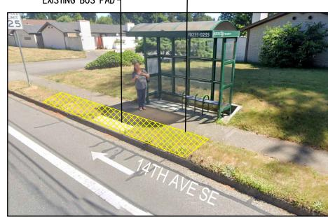
EXISTING CONDITION: BUS PAD WITH SHELTER, SIDEWALK, AND 3' WIDE PLANTER STRIP.
