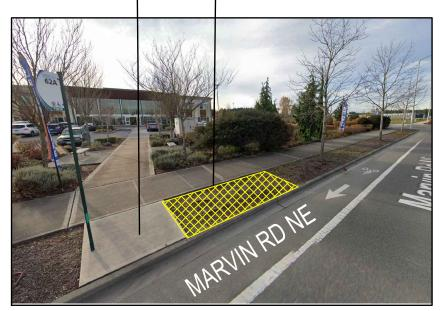
EXISTING CONDITION: BUS STOP (APPROX. 6'X6.5'), SIDEWALK, AND 6.5' PLANTER STRIP. INSTALL: LARGE PAD (APPROX. 18'X6.5'). MATCH EXISTING TOP OF CURB AND SIDEWALK. SEE SHEET L-DT-01 FOR LARGE PAD DETAIL. NOTE: LANDSCAPE IRRIGATION CONFLICT.
