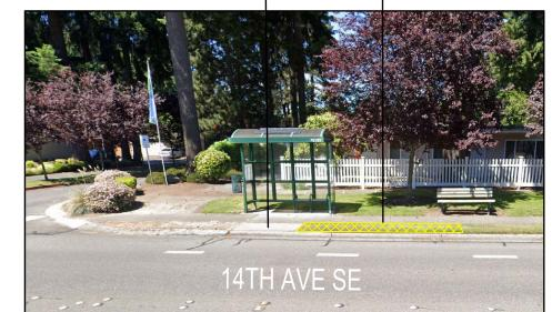
EXISTING CONDITION: BUS STOP WITH SHELTER WITH AN EXISTING PAD (APPROX. 3'X6'), SIDEWALK, AND 3' WIDE PLANTING
