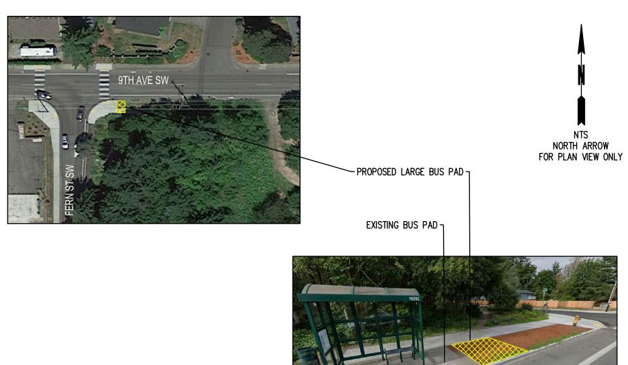
EXISTING CONDITION: BUS STOP WITH SHELTER, 16'X8' EXISTING PAD, SIDEWALK, AND 8' PLANTER STRIP. INSTALL: 8' WIDE REAR PAD (APPROX. 8'X8'). MATCH EXISTING TOP OF CURB AND SIDEWALK. SEE SHEET 0-DT-01 FOR LARGE PAD DETAIL. NOTE: NONE.
