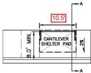
SHELTER ON SIDEWALK
